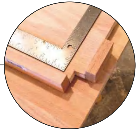
STEP 2. Next, notch corners to fit corner posts with an edge to meet the depth of the 2x2 corner post
